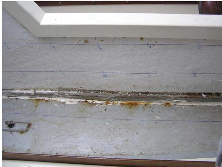
I discovered from discussion with Cornish Crabbers Ltd (now Select Yachts) that the ballast is made up of steel pressings set in a compound of slate dust and polyester resin. In BC each pressing is about 3 mm diameter and 1 mm thick. Several million of these pressings are used to make up the volume of ballast
