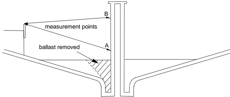
**Figure 1: Section through hull showing the ballast removed**
