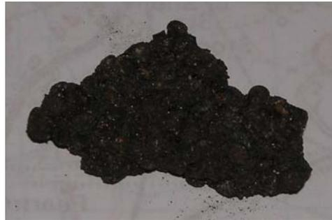
This clinker had formed expanding struts which had caused the centreboard case to be squeezed. In one place there was a void in the ballast about 50 mm long, 20 mm wide and high but the steel pressings around its surface had surprisingly not rusted.
