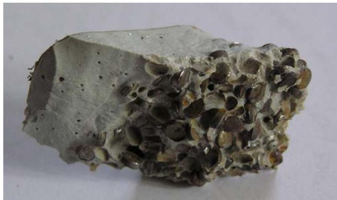
In order to understand my train of thought it is necessary to note that when sailing to windward the centreboard exerts large forces on the centreboard case (especially in strong winds). These forces may be sufficient to cause a crack to form between the fibre glass wall of the centreboard case and the ballast. Once such a crack has formed it provides access to sea water and oxygen. This allows the steel pressings to start to rust.
